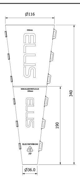
THE STUB TUBE IS ASSEMBLED WITH THE HOLD DOWN BOLT STANDING ON THE PLATE WASHER. THE TUBE IS LEFT IN PLACE WHILST THE SURROUNDING CONCRETE SETS. THE BOLT IS RETAINED BUT CAN MOVE DURING INSTALLATION OF ABOVE GROUND STEELWORK. POST INSTALLATION THE STUB TUBE CAN BE FILLED WITH GROUT.
