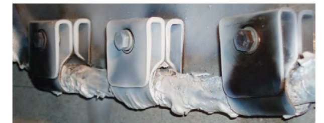
Phoenix clips have been fire tested in accordance with BS 589-1:2017
