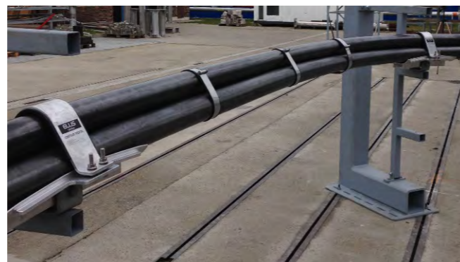
A photo of the short circuit test rig for Centaur Trefoil including Flexi-Straps (see page 28). Testing was carried out at ZKU Laboratories in Prague, CZ.
